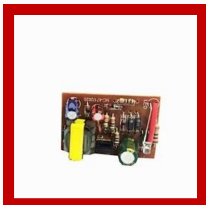
Printer Power Supply Board
